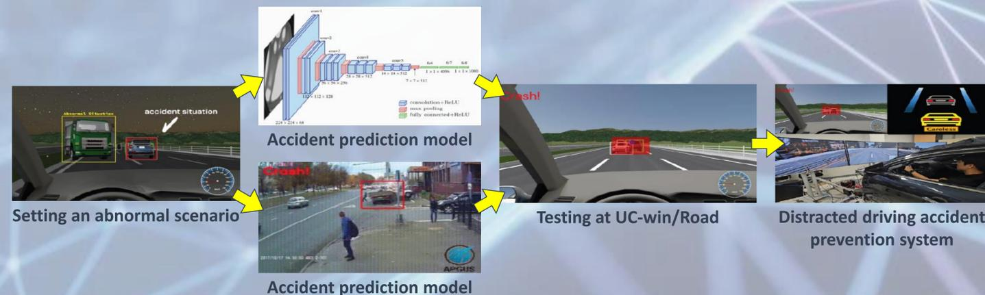
Utilize UC-Win/Road simulation to build and simulate anomaly scenarios. Predict risk situations and create bounding boxes. At the same time, a deep learning model is utilized to estimate the driver's gaze and project the 2D gaze point onto the uc-win screen to provide visual information to the driver. Finally, the GUI provides an appropriate warning by recognizing only the case where the estimated gaze point is not located in the bounding box in the predicted risk situation.
